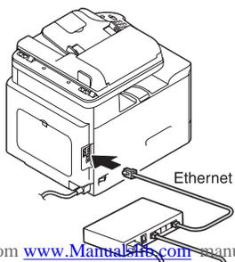
Connect an Ethernet cable or a USB cable as shown (Ethernet and USB cables are not included in this shipment).
